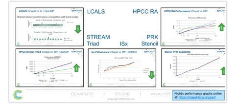
Chapel vs. MPI/OpenMP performance in recent talks, demonstrating that Chapel is increasingly competitive for local computations (LCALS), embarrassingly parallel computations (stream), random fine-grain communication (RA), stencil communications (Stencil PRK), and bucket exchange patterns (ISx). The distributed memory timings here are on 2×18-core compute nodes (so 256 locales = 256\*36 cores)
